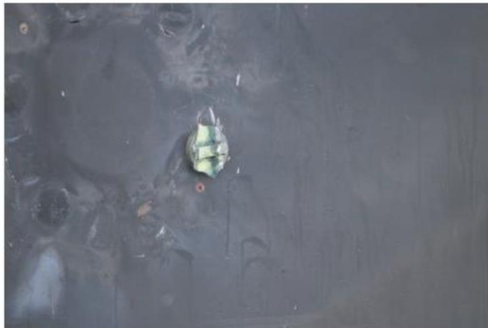
7714 - This is the view of the remnants of a removed limpet mine's placement, location, and damage sustained from a limpet mine attack, on the starboard side of motor vessel M/T Kokuka Courageous, while operating in the Gulf of Oman, June 13. A limpet mine is attached to a vessel via magnet and/or nails. The holes seen were created by nails used to hold the mine in place.
