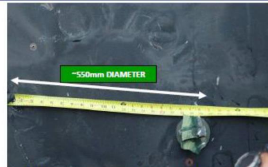
(U) Measurements are consistent with reported diameter of Iranian Extra-Large limpet mine
