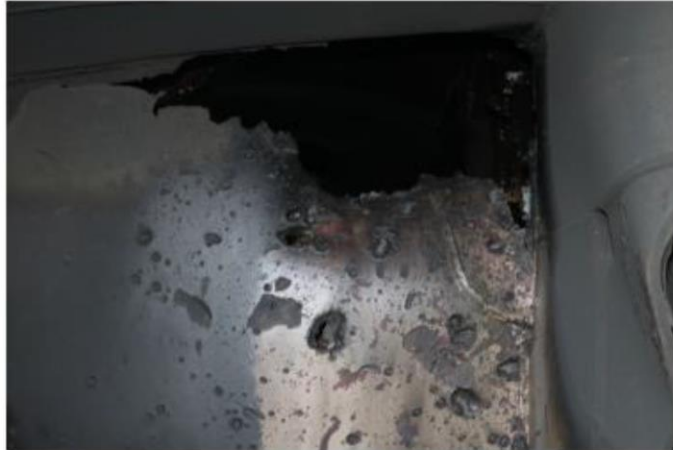
7729 - This photo is a view of internal hull penetration/blast damage sustained from a limpet mine attack on the starboard side of motor vessel M/T Kokuka Courageous, while operating in the Gulf of Oman, June 13.
