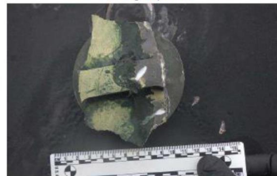
(U) Magnet 3.5" diameter; aluminum, composite remnants
