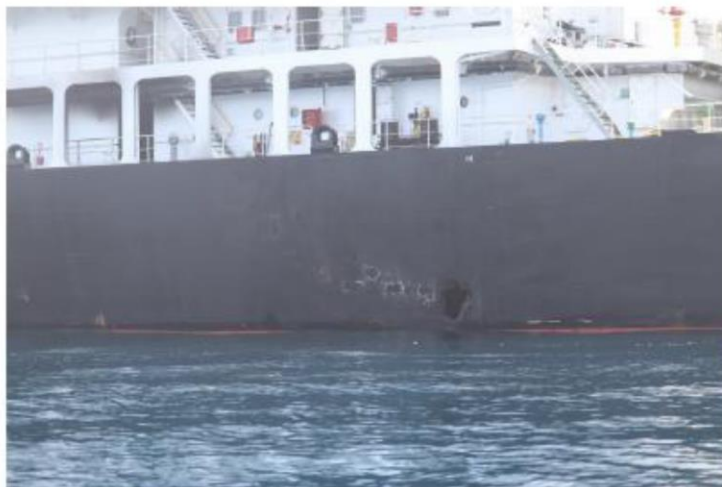
7710 – This is a view of hull penetration/blast damage on the starboard side of motor vessel M/T Kokuka Courageous, which was sustained from a limpet mine attack while operating in the Gulf of Oman, on June 13th.
