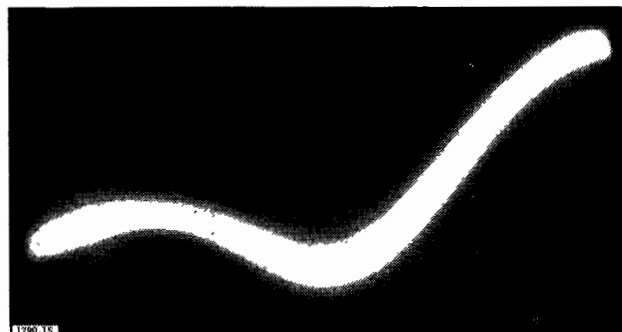
Figure 15. Off-axis arc in DCX. About three feet of arc are visible
