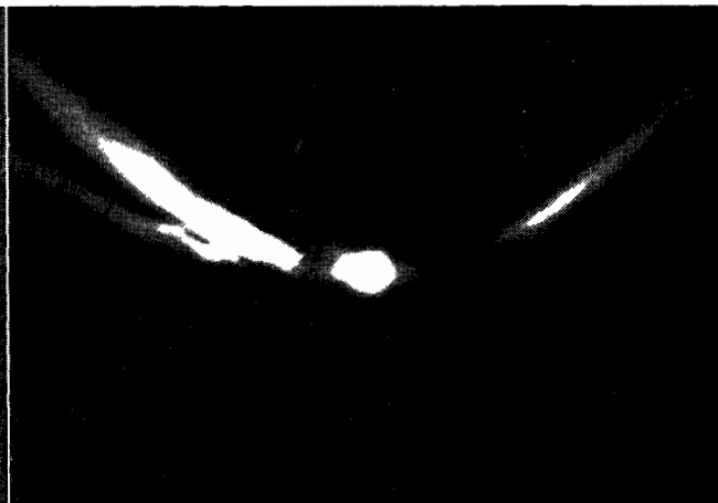
Figure 13. Ion energy analysis by Thomson method. B = 1500 g; E = 1850 v/cm; V_p = 40 kv; P_{D_2} = 0.04 mm Hg; photographs for two different directions of H^- . 7 pulse discharges, D^+ parabola upwards (slightly blackened), D^- parabola downwards
