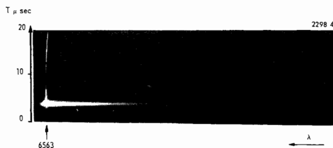
Figure 4. Streak photograph of the spectrum of a hydrogen discharge
