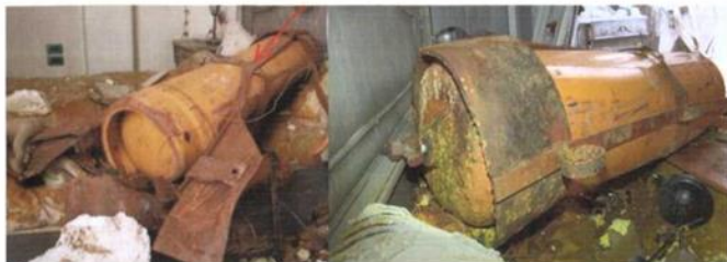
The cylinder should have more flattened form for the flat penetration. The stabilizing fins, valve and other elements should have more significant deformation or be absent
