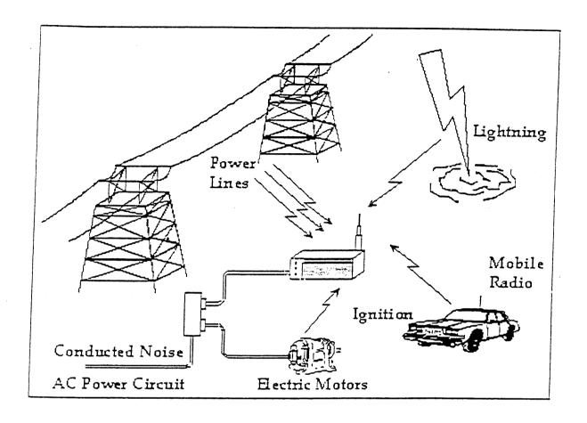
Figure (2): Some factors affecting Electromagnetic Compatibility
