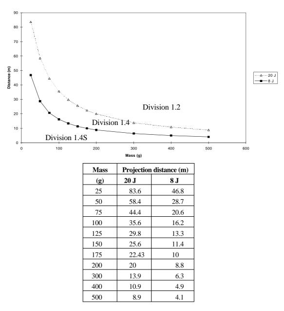
Example data for metallic projections with a kinetic energy of 20 J and 8 J
