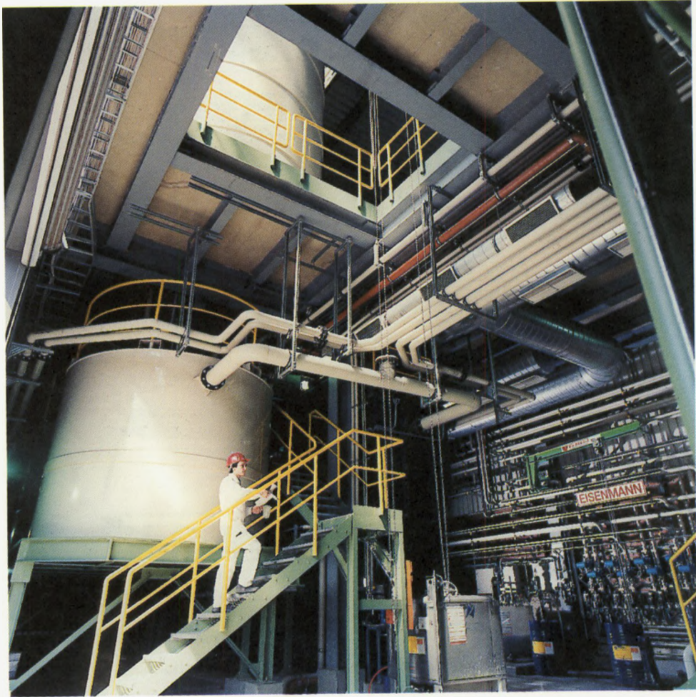
Photo 22: Closed loop water recycling
