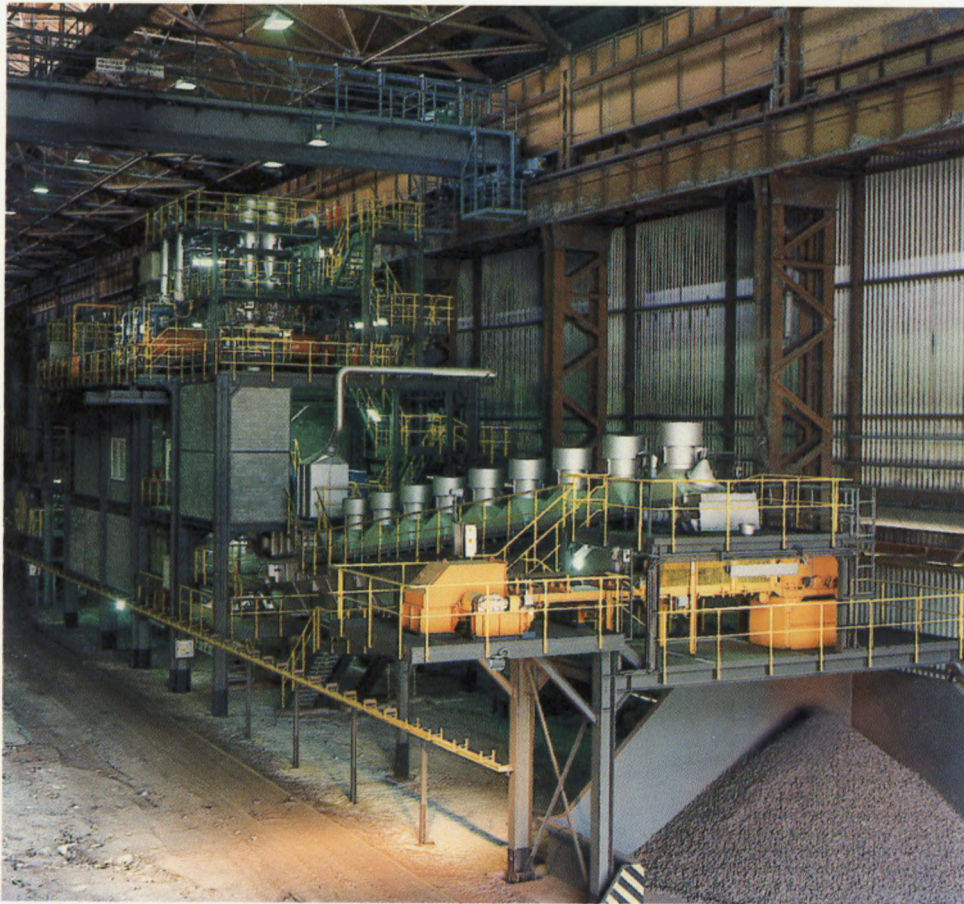
Photo 12: Pelletisation of steel plant dust
