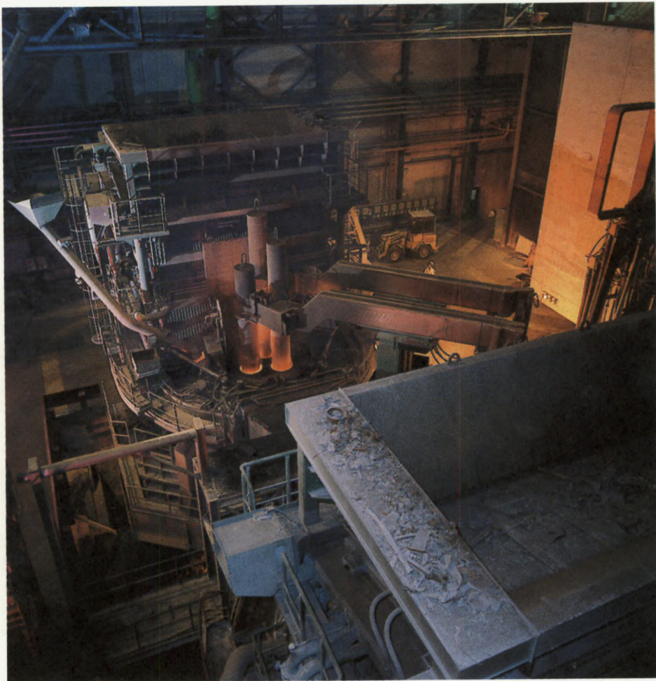
Photo 14: Electric arc steelmaking — example of a twin shaft furnace
