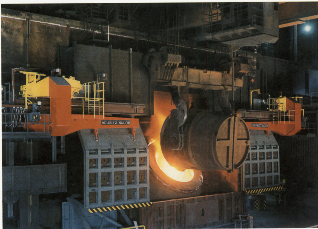
Photo 10: Charging hot metal into a BOS vessel
