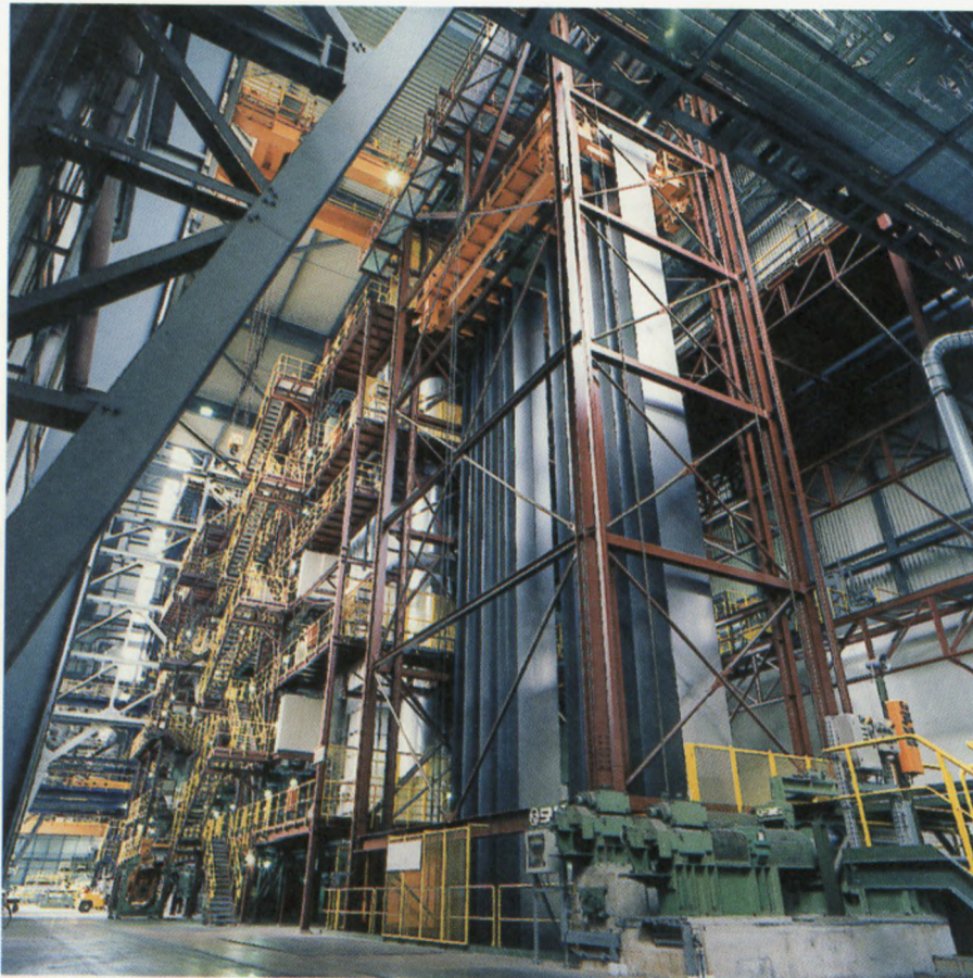
Photo 21: A continuous annealing line for steel sheet
