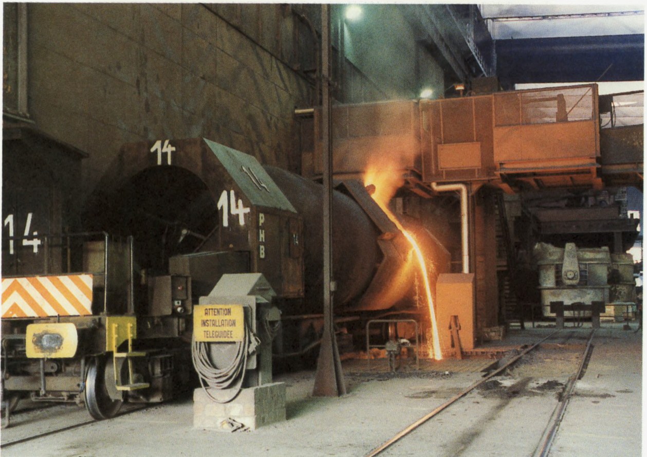
Photos 8 and 9: Case study of improving emissions from a hot metal torpedo ladle with CO 2 blanketing
