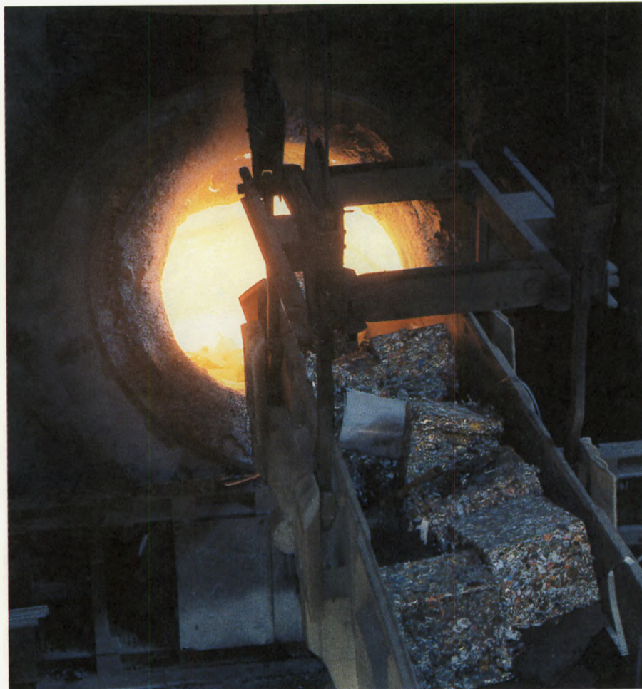
Photo 11: Charging recycled steel into a BOS vessel
