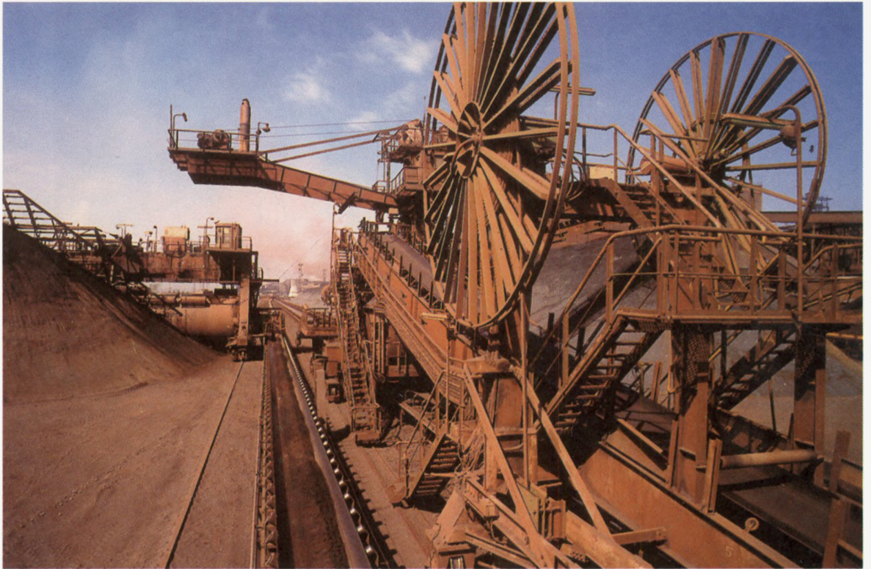
Photo 2: Reclamation of iron ore from iron ore beds at the steelworks
