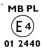
The headlamp bearing the above approval mark is a headlamp incorporating a lens of plastic material which has been approved in the Netherlands (E 4) under approval number 01 2440. The approval number indicates that the approval was granted in accordance with the requirements of this Regulation, as amended by the 01 series of amendments.
