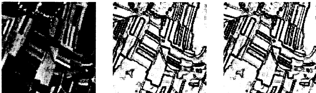
Figure 5 Grey level image (left), gradient magnitude image (middle), thresholded gradient magnitude image (right)
