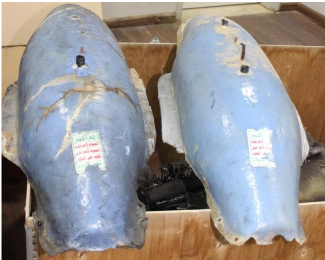
Figure 12.6 Possible external fuel tanks for the UAV-X
