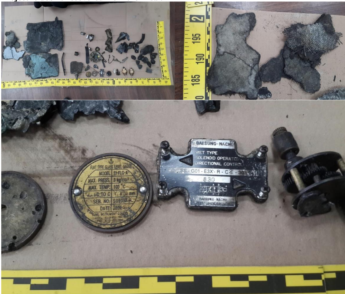
Figure 15.5 Projectile debris recovered from the Arsan
