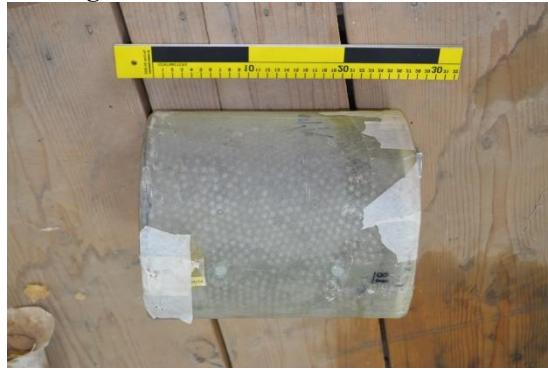
Figure 12.5 Warhead of explosives mixed with ball bearings recovered from UAV-X debris
