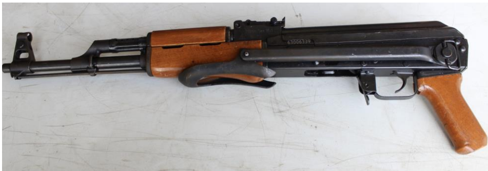
Figure 16.5 Close-up Type 56-1 assault rifle, showing the underfolding steel shoulder stock
