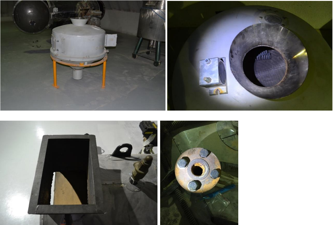
Figure 14.4 Metal container with a metal mesh screen
