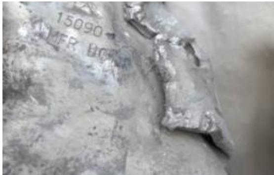
Figure 33.G.3 Fragmentation from Paveway guidance unit
