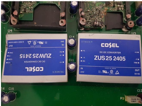
Figure 13.2 ZUS25 2415 and ZUS25 2405 DC-DC power converters
