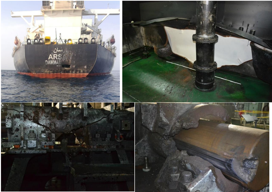
Figure 15.4 Damage on the Arsan
