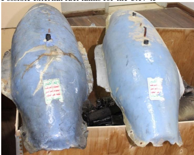
Figure 12.6 Possible external fuel tanks for the UAV-X
