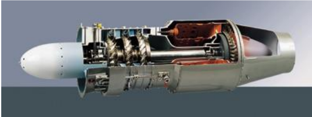
Figure 11.5 Features of TRI-60-2
