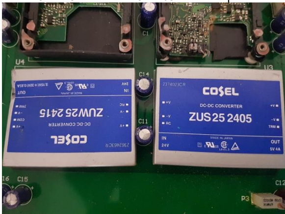
Figure 13.2 ZUS25 2415 and ZUS25 2405 DC-DC power converters
