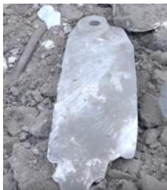
Figure 33.G.1 Rear wing of Paveway guidance unit
