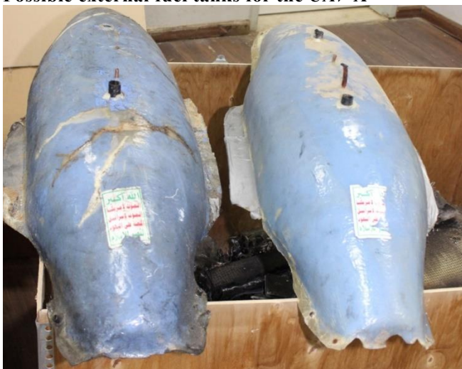
Figure 12.6 Possible external fuel tanks for the UAV-X
