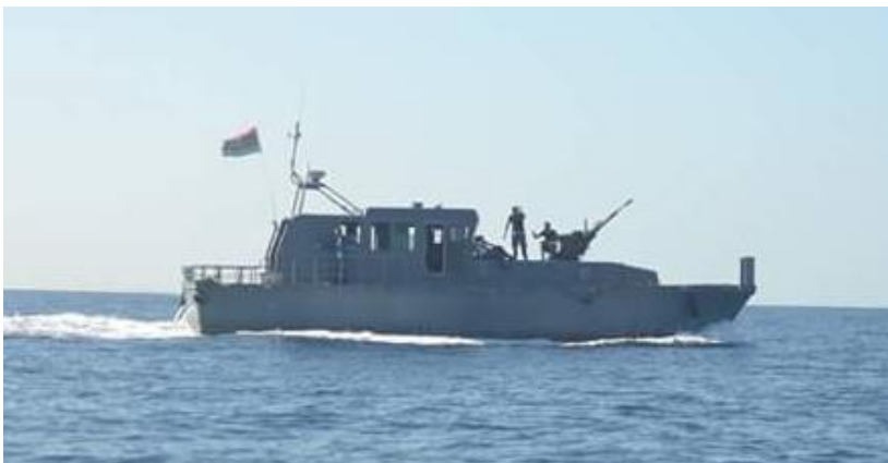
Picture 26 Probably a former pilot boat modified into a patrol boat. On the bow, an anti-aircraft 23mm machine gun
