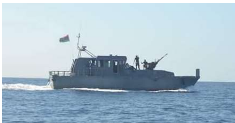
Picture 26 Probably a former pilot boat modified into a patrol boat. On the bow, an anti-aircraft 23mm machine
