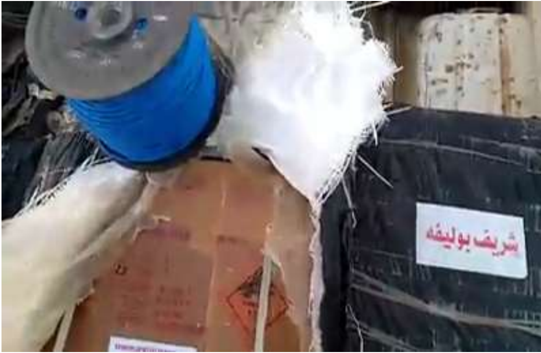
Picture 15 Detonating cord produced by Kapeks Ltd. (One of the boxes featuring the caution symbol for explosives and an unpacked roll of detonating cord above the box)
