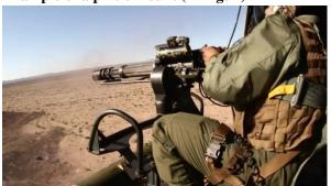
Figure A.58.12 **Example of a pintle mount (7.62mm MMG)**<sup>45</sup>
