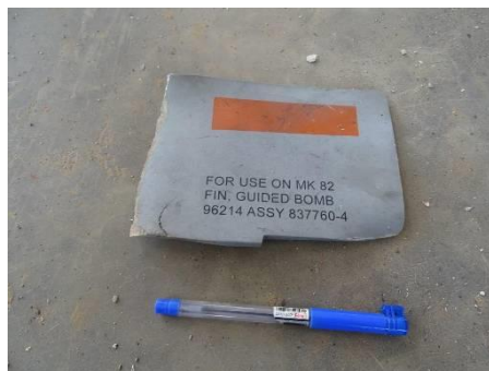
Figure B.60.6 Paveway IV laser guidance fin 20
