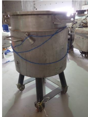
Figure D.36.4 Storage or transfer vessel
