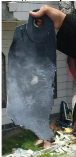
Figure D.60.2 Post-explosion guidance wing from a Paveway laser guidance system
