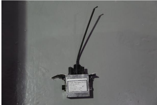
Figure B.38.7 IMG-3009: Full Duplex Multi-Frequency Data Link
