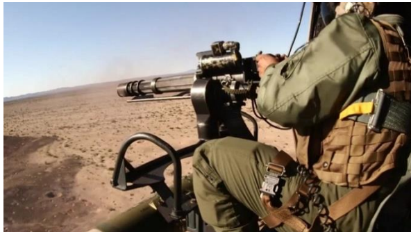
Figure A.58.11 Example of a pintle mount (minigun) 44
