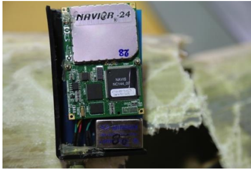
Figure B.38.4 IMG-3028 NAVIOR Satellite Compass NAVIS NC144_02
