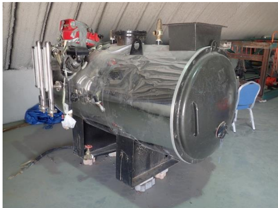
Figure D.36.7 Pressure vessel
