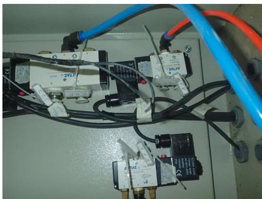
Figure D.36.24 Solenoid Valves Models 4V210-08 / 4V110-15 (Partial Traced: > IR)
