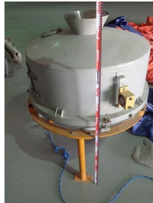
Figure D.36.8 Heating vessel
