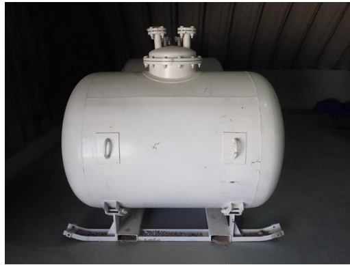
Figure D.36.10 Field storage tanks for liquid bi-propellant oxidiser
