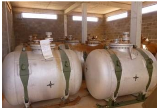
Figure X Scud oxidizer field storage tank a
