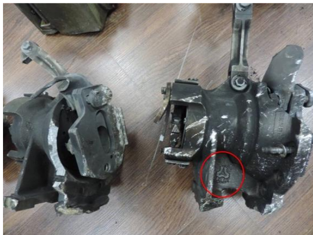
Figure 36.10 Jet vane housing with Shahid Bagheri Industries logo markings
