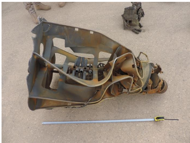
Figure 35.2 SCUD C type sub munition warhead (Ta'if, 26 July 2017) 3
