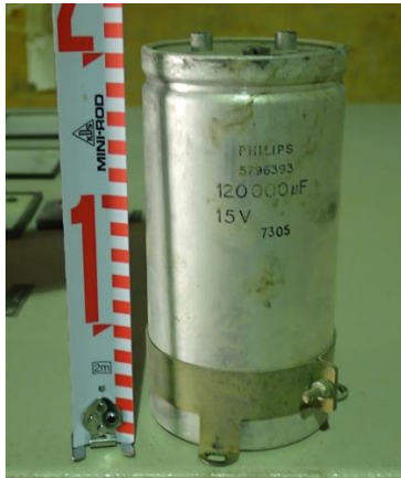
Figure D.36.19 12000UF 15V Capacitor
