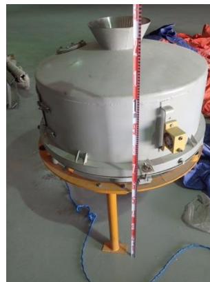
Figure D.36.8 Heating vessel
