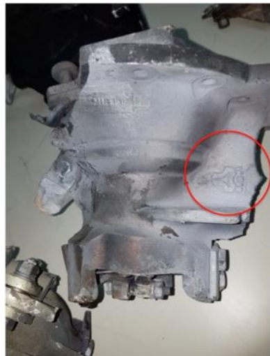
Figure 36.8 Jet vane housing with Shahid Bakeri Industries logo markings
