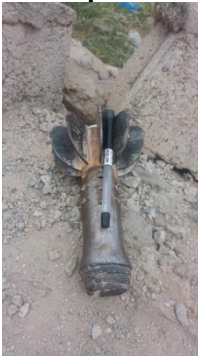
Figure A.64.1 Post explosion - Tail fragment
