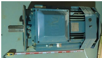
Figure D.36.17 M3KP 224 Smb 4 Motor
