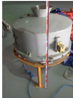
Figure D.36.8 Heating vessel
