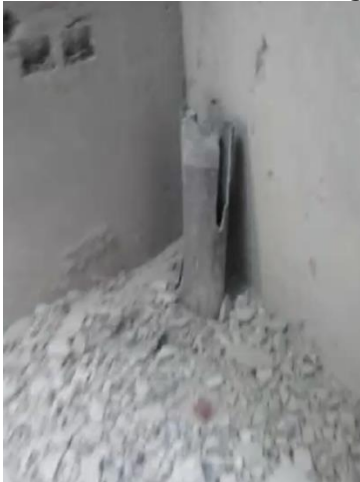
Figure B.64.1 120mm HE mortar bomb fragment
