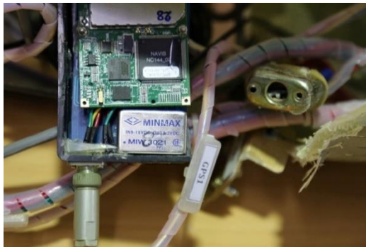
Figure B.38.3 IMG-3029: DC Output Converter MIW 3021
