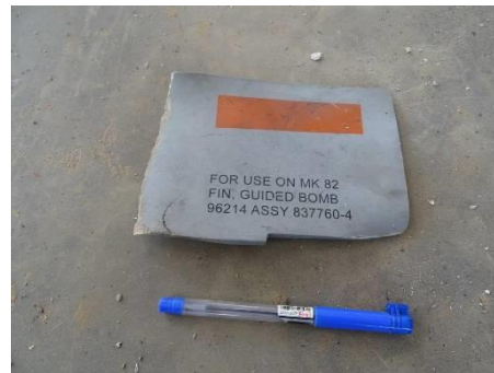
Figure B.60.6 Paveway IV laser guidance fin 20
