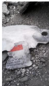
Figure F.60.5 Guidance fin and component from a Paveway laser guidance system
