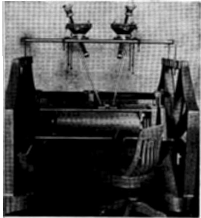
Figure 84. The 1960 Orthophotoscope with Kelsh-type projectors
