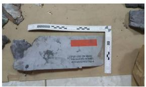
(e) One fragment has the shape profile, and falls within the dimensional parameters, of a fragment from the wing of a guidance unit for a HE aircraft bomb (figure 49.D.8 and 49.D.9).
