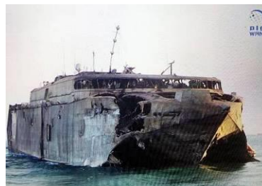
Figure 13.3 Impact point of ASM on Starboard Bow
