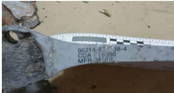
Figure 49.D.10 GBU-12 PAVEWAY II guidance unit wing fragment showing manufacturers CAGE code 3FU05 302
