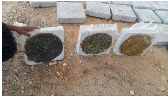
Figure 43.8 “Rock” IED with Minimal Metal Pressure Plate, Location TBC (10 Jun 2016)
