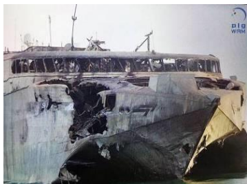
Figure 13.2 Impact point of ASM on Starboard Bow
