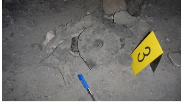
Figure 49.D.9 GBU-12 PAVEWAY II guidance unit wing fragment in situ 301
