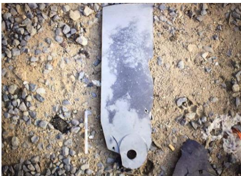
Figure 49.C.3 Probable GBU-12 PAVEWAY II guidance unit rear wing 264
