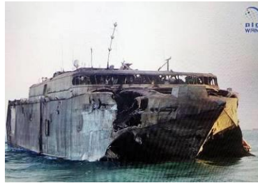
Figure 13.3 Impact point of ASM on Starboard Bow
