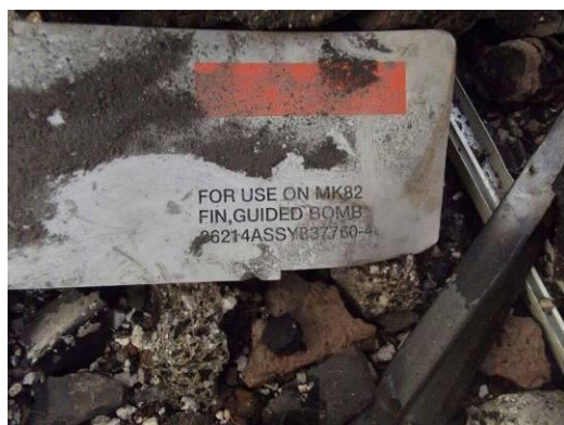
Figure 49.D.6 GBU-12 PAVEWAY II guidance unit fin fragment in situ 299
