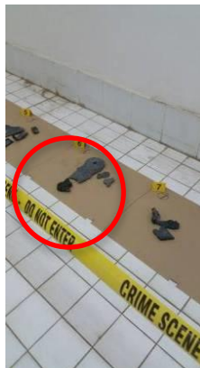
Figure 49.D.11 GBU-12 PAVEWAY II guidance unit wing fragment
