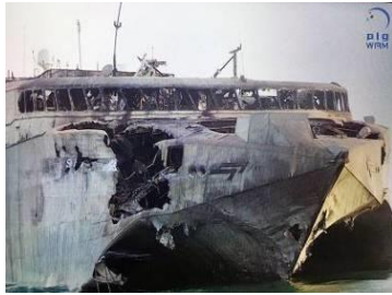
Figure 13.2 Impact point of ASM on Starboard Bow
