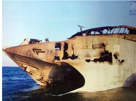
Figure 13.5 Fire damage to aluminium superstructure on Port Bow
