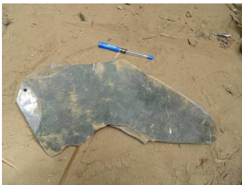
Figure 49.A.2 Rear fin from PAVEWAY terminal guidance unit 216
