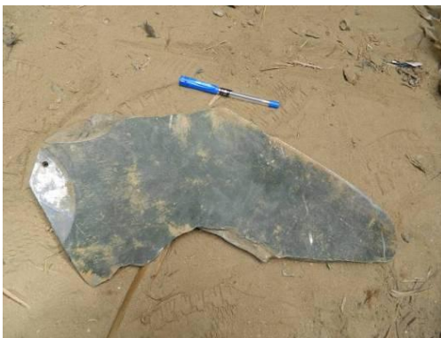
Figure 49.A.2 Rear fin from PAVEWAY terminal guidance unit 216
