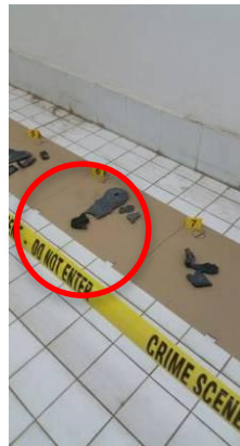
Figure 49.D.11 GBU-12 PAVEWAY II guidance unit wing fragment
