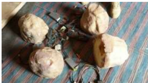
Figure 43.2 'Rock' IED with possible Passive Infra Red (PIR) initiator, Saleh, Ma'rib (30 Oct 2016)
