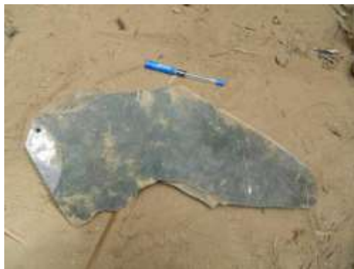
Figure 49.A.2 Rear fin from PAVEWAY terminal guidance unit 216
