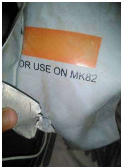
Figure 49.B.5 Post-explosion adapter flange from a Paveway laser guidance system
