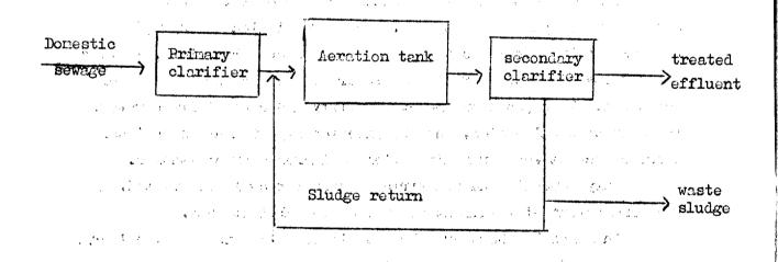
.. Fig.1. The Activated Sludge Process.
