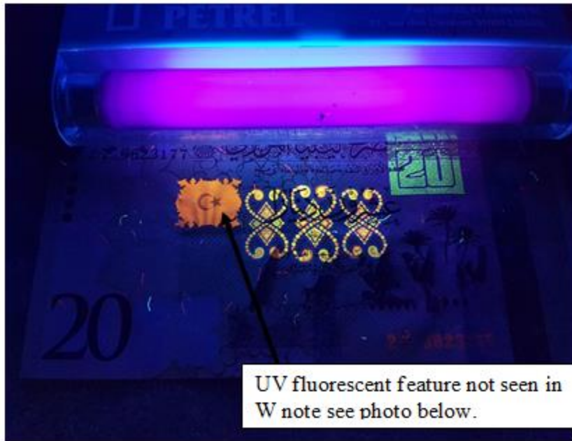
Photo 5: UV features on front of alternative banknote
