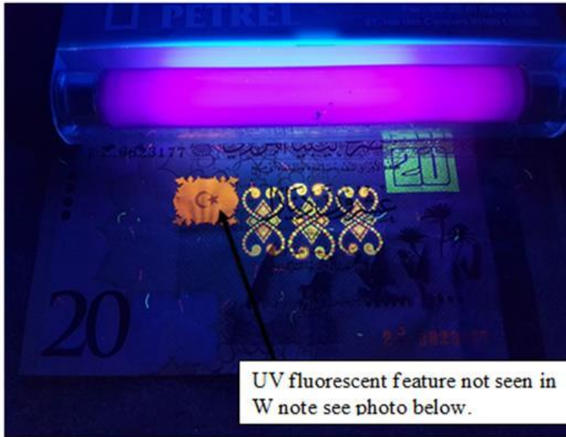
Photo 5: UV features on front of alternative banknote
