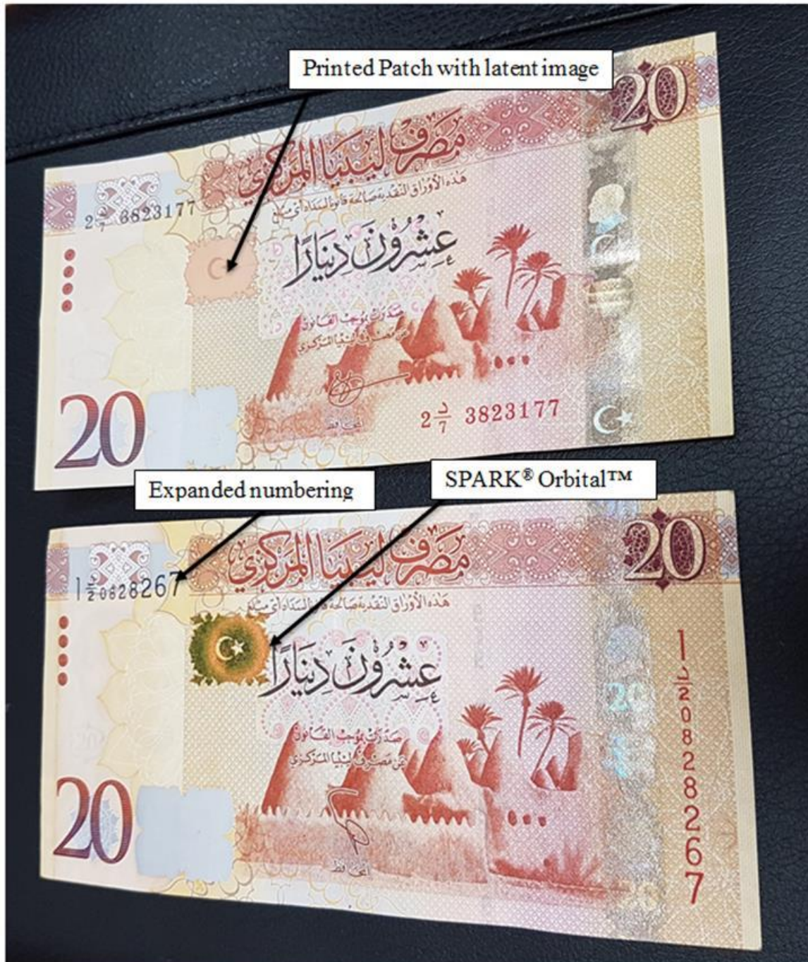
Photograph 2: front side, oblique angle - alternative banknote (top) and original banknote (bottom)
