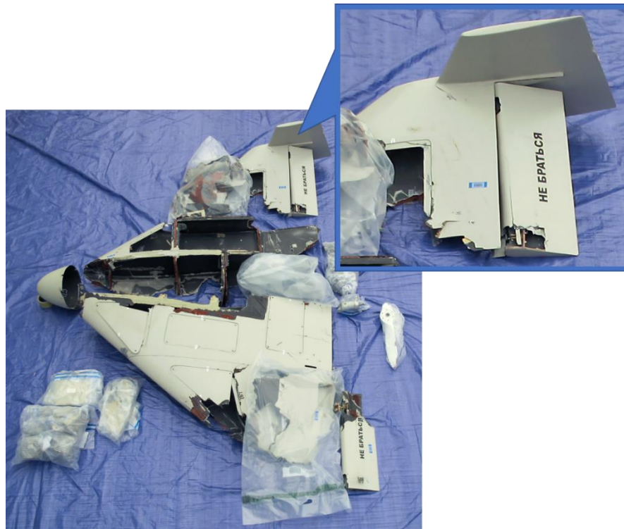
Figure 15: Shahed-136 system loaned to the UK by Ukraine with highlighted wing stabilizer
