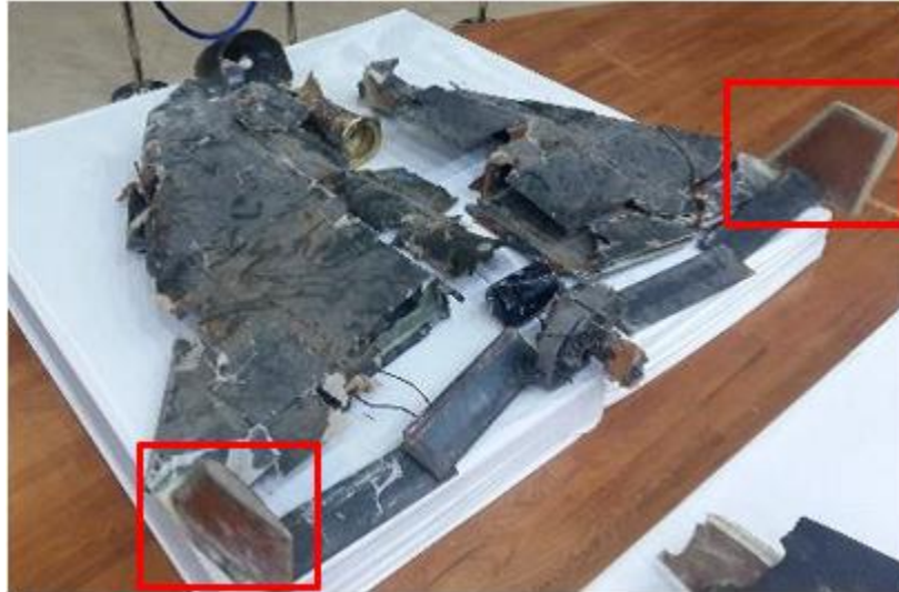
Figure 11: Shahed-131 debris shown in KSA (2019) with highlighted wing stabilizers
